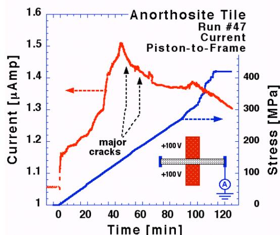
This experiment still left us with some uncertainty as to how much current was surface current, flowing along the surface of the rock. We therefore added guard electrodes on both sides of the tile halfway between the pistons and the frame made of 6.3 mm wide Cu stripes. The results indicate that the guard electrodes captured  $\leq$ 30% of the current flowing from the pistons to the periphery, while  $\geq$ 70% of the current passed through the interior (Freund et al. 2004).
