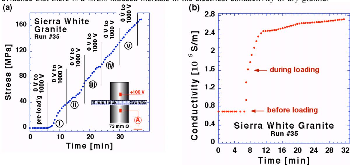
Figure 5a: Loading curve and b: stress-induced changes in conductivity of an air-dry granite slab.
