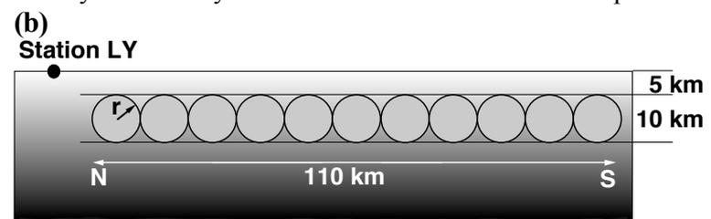
Figure 4a: Taiwan magnetometer network with rectangular “source volume” used for modeling the ground current. Solid line: approximate location of the Chelungpu fault. b: Cross section through the assumed ground conductor.
