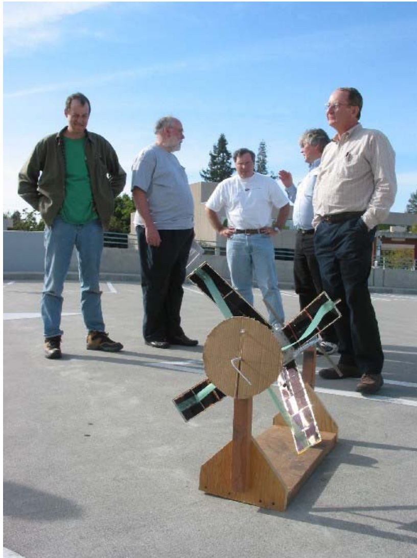
QuakeSat and team performing the solar array rotisserie testing in the office parking lot.
