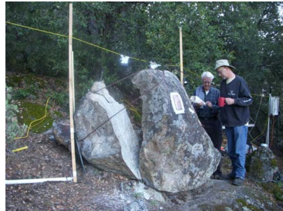
The rock finally broke into 4 major pieces after 9 hrs
