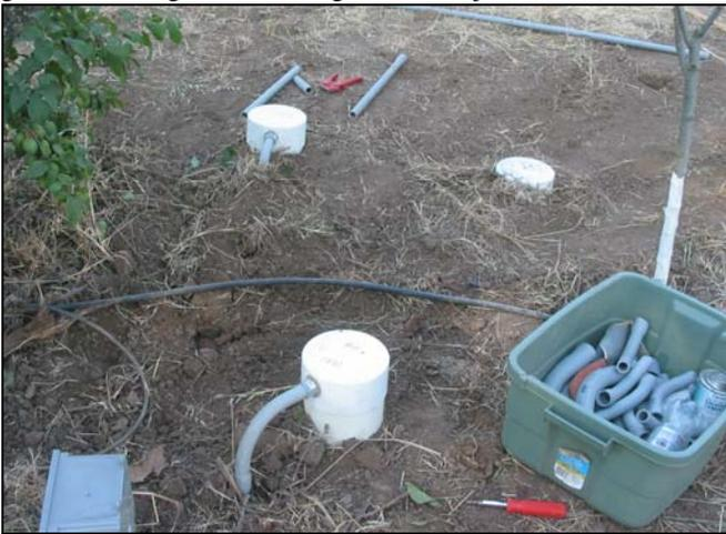
**Buried Magnetometers and Junction Box**
